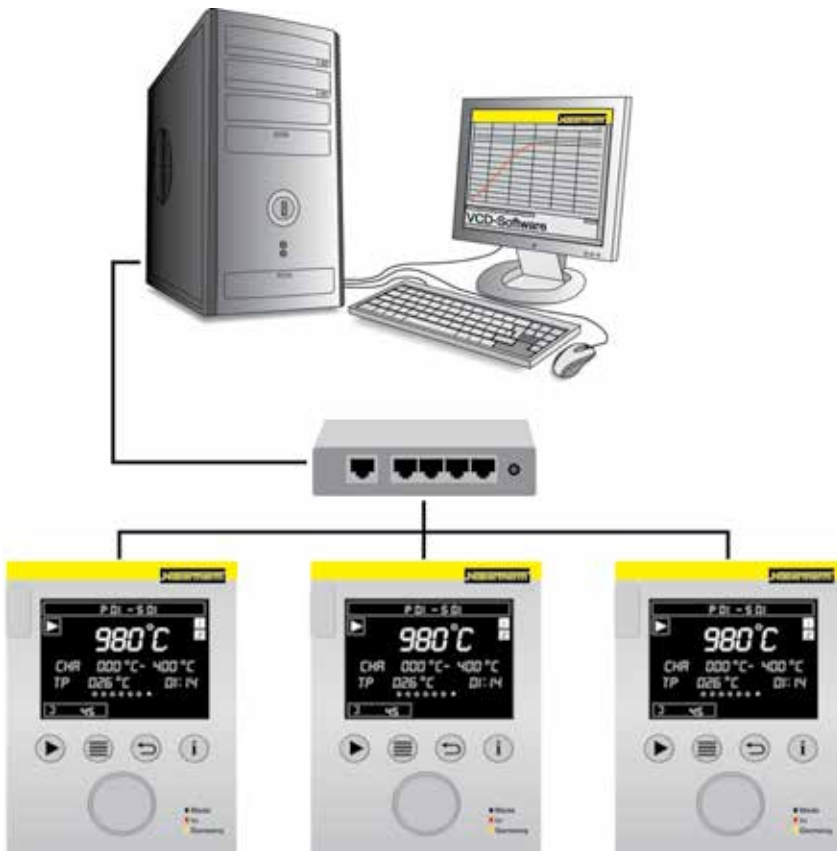
Example lay-out with 3 furnaces
