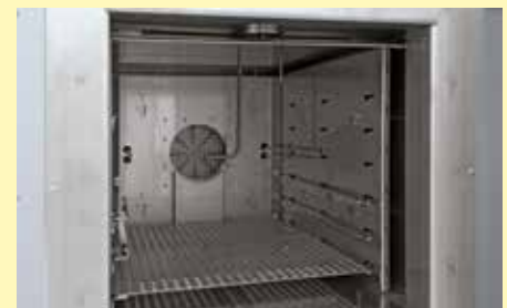
Interior with metal shelf, thermocouples and pressure monitoring
