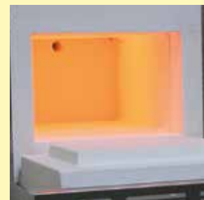
Muffle heated from four sides
