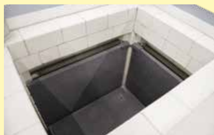
Sides and floor lined with silicon carbide tiles as protection for pit-type furnace S 73/HS
