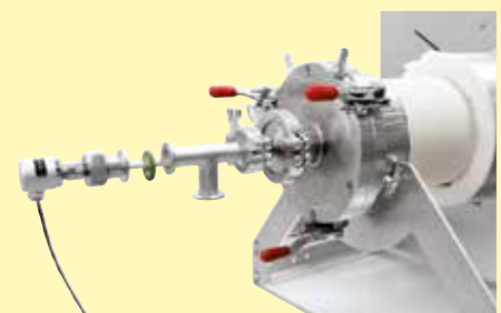
Thermocouple for charge control
