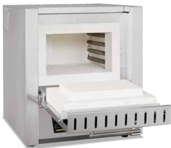
Muffle furnace L 9/13 with flap door
